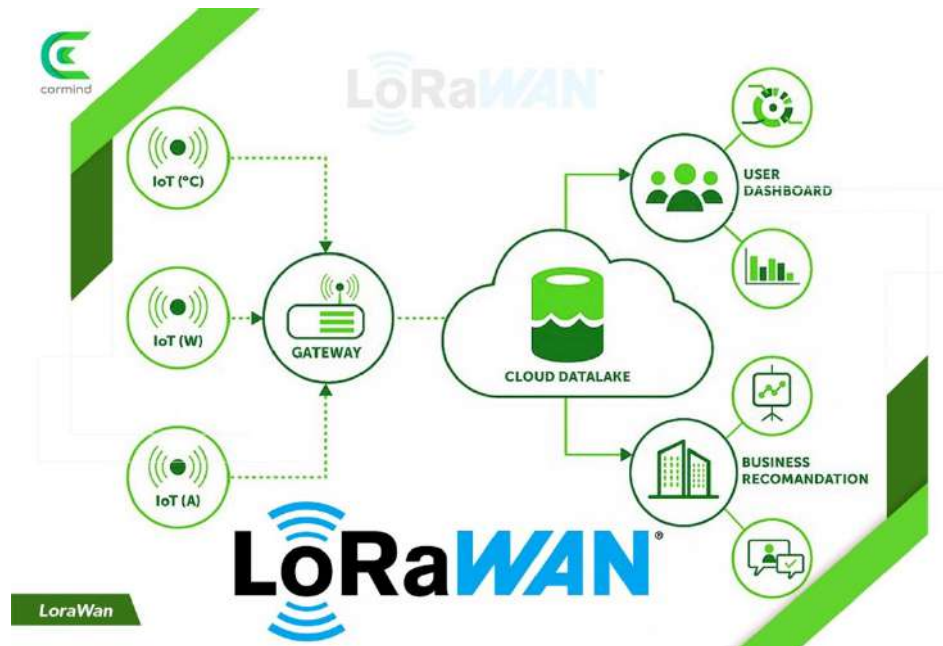
Fig. 1: Architecture of LoRaWAN network [2]
