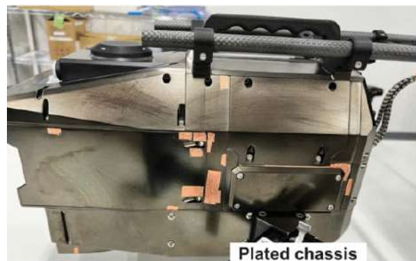
Figure 7: [1] Conductive plating for UAV chassis
