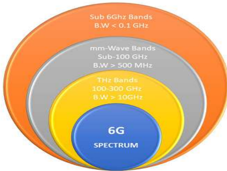
Fig. 3: The frequency spectrum in 6G communication.(3)
