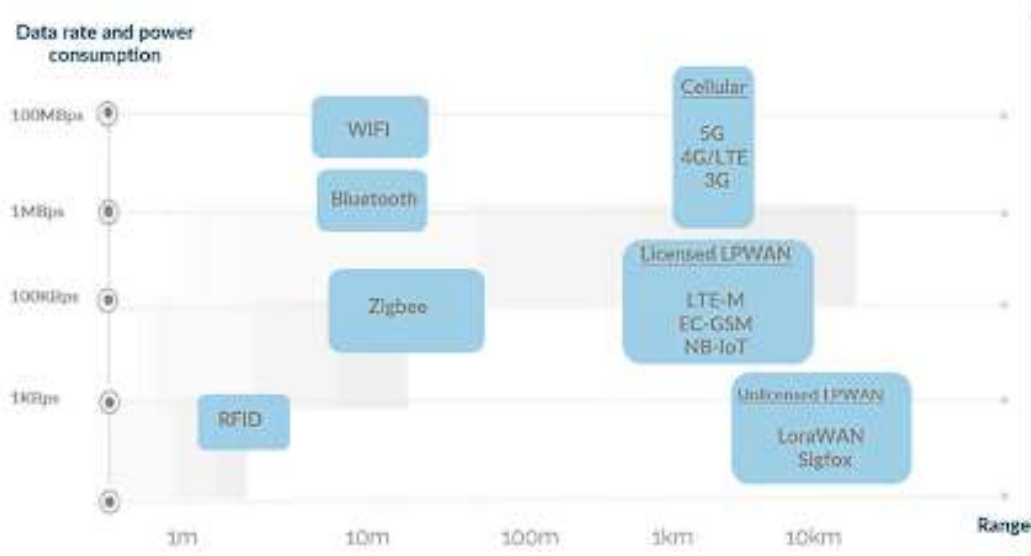
Fig. 1: IoT wireless technologies range and bandwidth,
