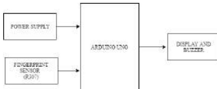
Fig. 1: . Block diagram of verification unit
