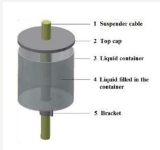
Figure 1: Proposed Ring Shaped Tuned Liquid Damper (RSTLD) for suspender cables
