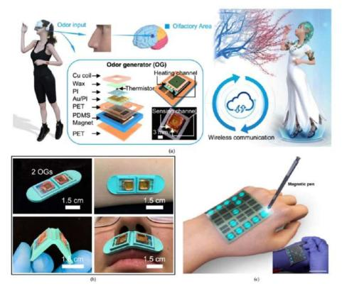
Fig. 2: E-skins for virtual olfactory experience and magnetoperception. (a) and (b) Architectures of the olfaction interfaces. (a) Schematic diagram of the olfaction interface and its application in VR experience. The schematic illustration in the frame shows an exploded view of the odor generators. (b) Optical images of the olfaction interface mounted onto a human, Springer Nature. (c) Schematic of a  $5 \times 5$  magneto-interactive display array[3]
