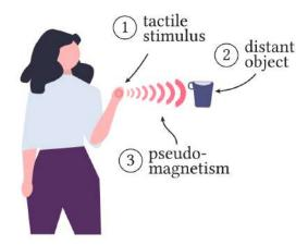
Fig. 2: Core principles of Haptic Magnetism: tactile stimulation, dynamic distance-based feedback, and pseudo-magnetic interactions[6]
